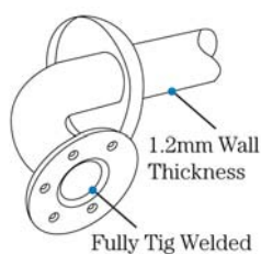
Standard Grabrail Bend with TIG Welded Fixing Flange
